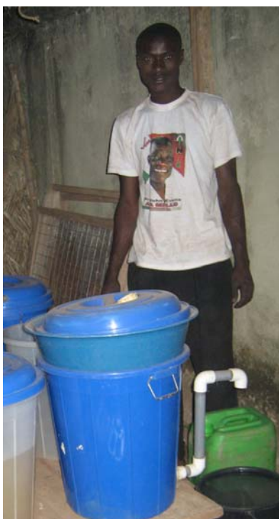
Figure 8: Local Plastic Design Biosand Filter
