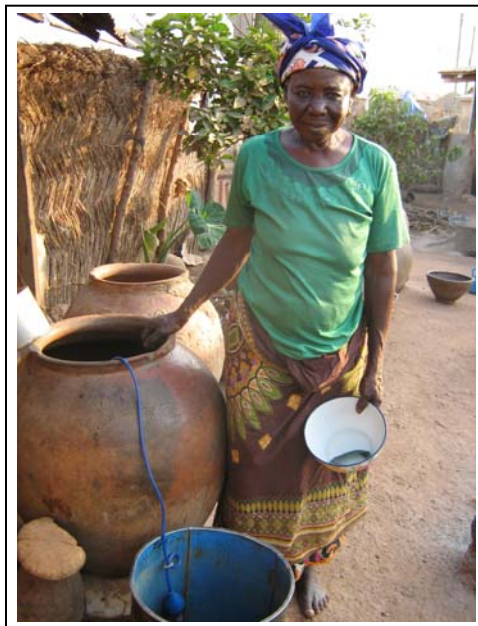
Figure 6: Woman with large ceramic pot used as upper container for siphon filter
